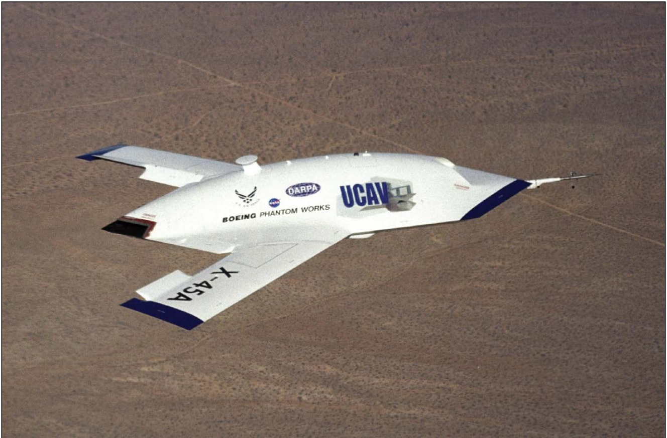
The X-45 Unmanned Combat Air Vehicle technology demonstrator that is eventually intended to fly high-risk air combat missions.
